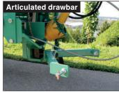
With the standard draw bar the machine can be appended to the tractor with low hitch and twistable towing bracket. The articulated drawbar appended to the tractor in the lower link. The machine follows exactly to the towing vehicle track. For lines with a narrow headland the articulated drawbar is also available with wide-angle PTO shaft. There is a 80 °turning angle possible while running the PTO. All hitches are delivered with a Walterscheid PTO shaft with friction clutch.
