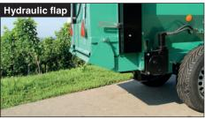
The hydraulic flap is closing the material throw-off and prevents material falling out on the street.
