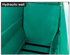
The scraper floor is driven hydraulically. All types are also available with a hydraulically pushing wall. This wall is activated by a valve and moves automatically with the adjusted speed in both directions.
