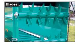
The blades mounted on the Spreading roller chuff long material like straw or horse manure. In conjunction with machines using a hydraulic driven wall, it is also possible to chuff and spread straw square bales.
